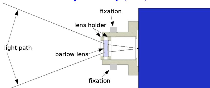
Fig 2. The incoming light (from left) reaches the barlow lens and is focused on the detector. The lens is fixed by two lens holders to ensure that the lens is at the right distance from the detector. The fixation is used to mount the optical system at the output of the O.L.T.
