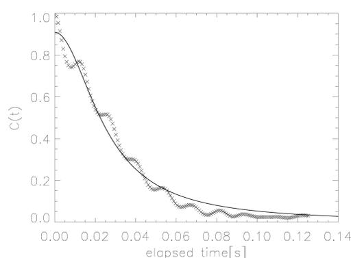
Fig 3. Time-only autocorrelation function  $C(t)$  of the stellar speckle pattern. The crosses denote the values derived from the observation of Arcturus and the line denotes the fit to the theoretical model.
