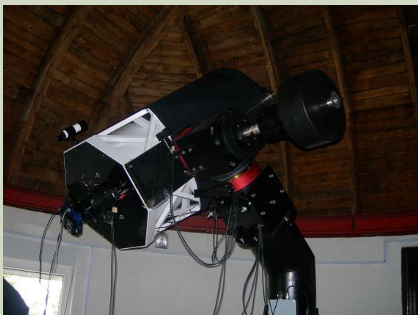
Figure 1: Telescope Cassegrain 60cm, ASV
